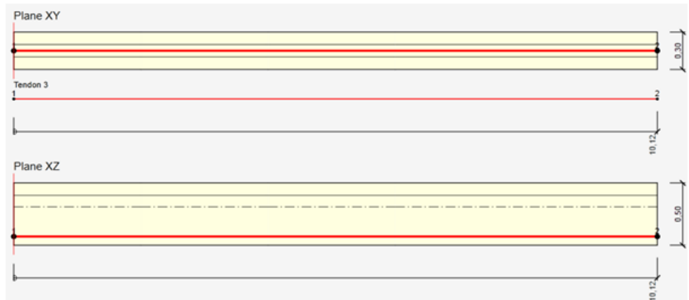
Figure 3.37: Example 1 : Design member uncoiled views in planes XY and XZ including straight tendon
