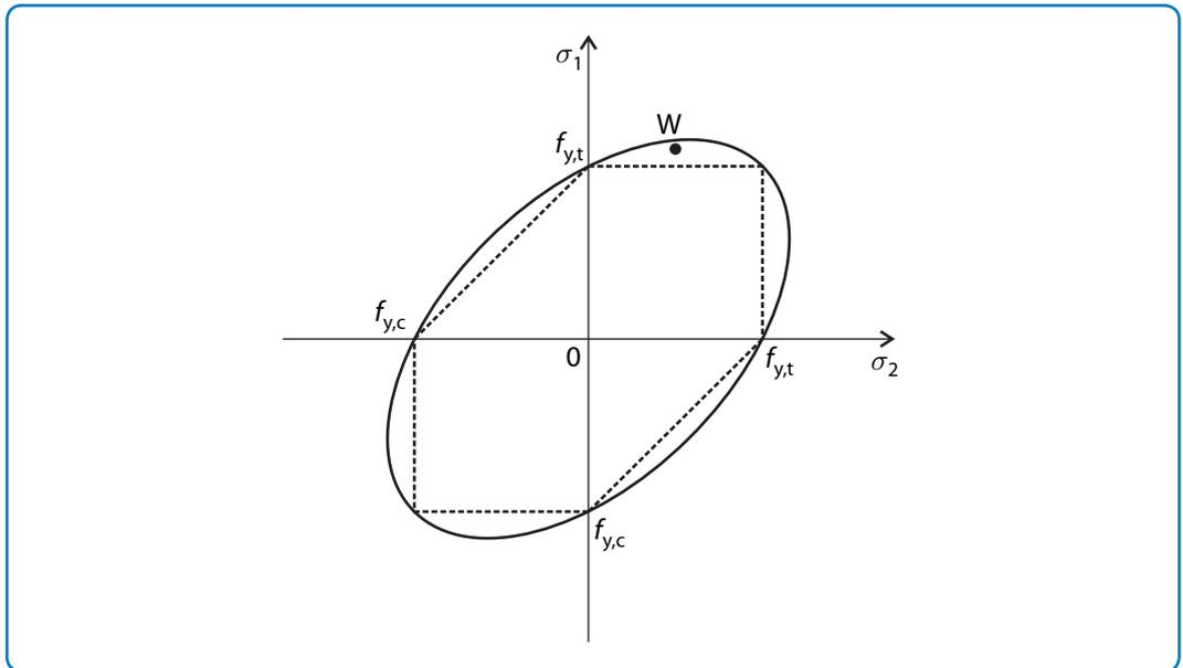
**Figure 2:** Von Mises and Drucker-Prager (solid line) and Tresca and Mohr-Coulomb (dashed line) plastic models in plane and considering equal plastic strength in tension and pressure. W is the working point of this verification example.
